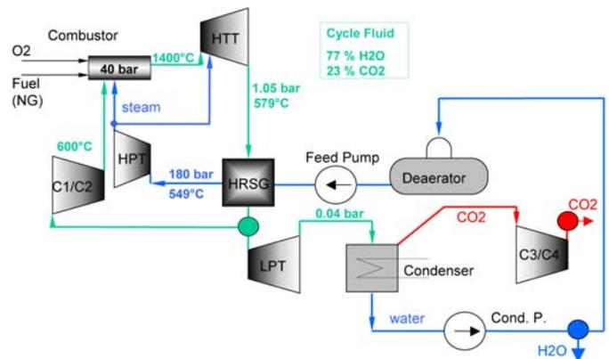
**Fig. 1:** Principle flow scheme of the basic Graz Cycle power plant
