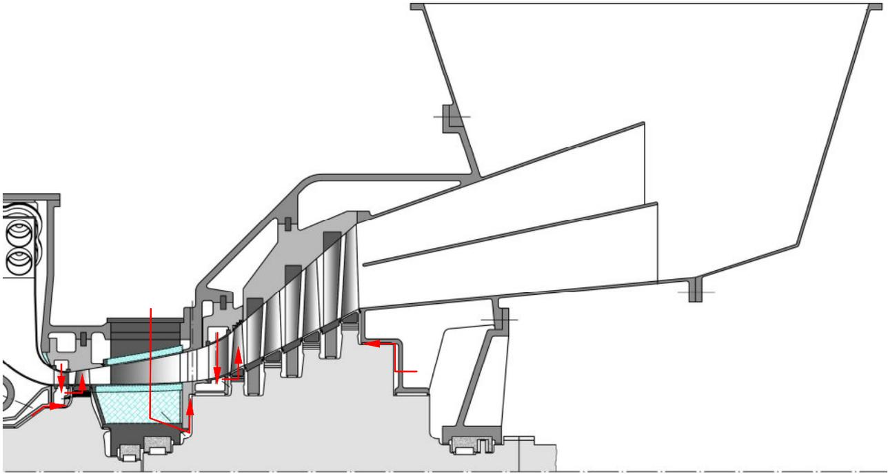
**Fig. 8:** Design of transonic one-stage HTTC and 60 Hz HTTP
