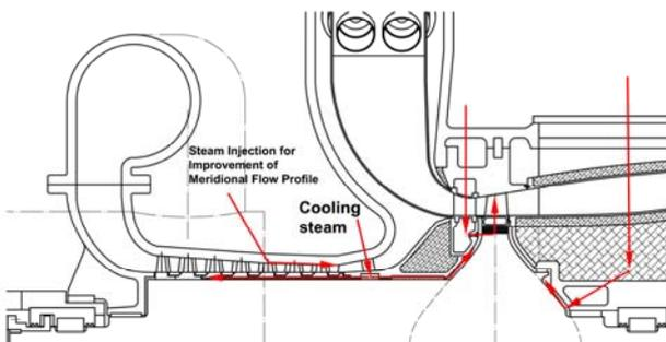
Figure 5 - Details of transonic stage of HTTC with steam cooling by ICS.
