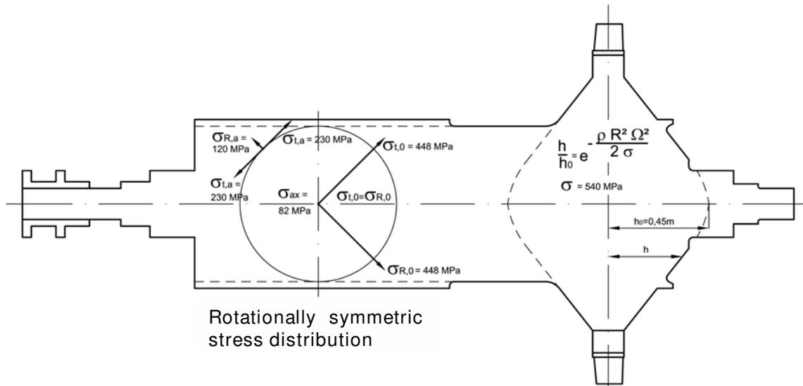
Figure 7 - C2-HTTC shaft with analytic solutions for three-dimensional stress indicated
