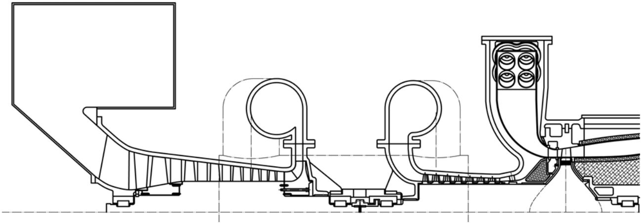
Figure 3 - Design of high speed shaft consisting of compressors C1 and C2 and compressor turbine HTTC
