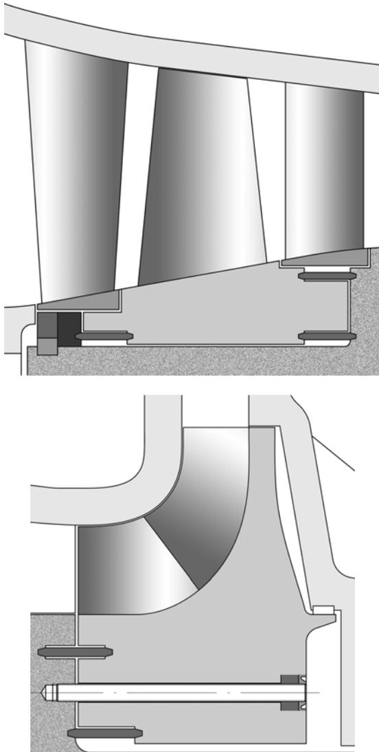
Figure 9 - Details of the first and last stage of compressor C1
