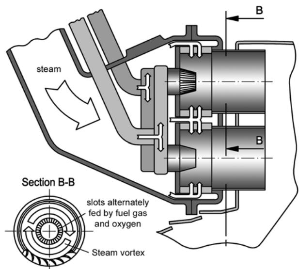
Figure 6 - Graz Cycle combustor consisting of 6 quadruples of 4 burners each in circumference
