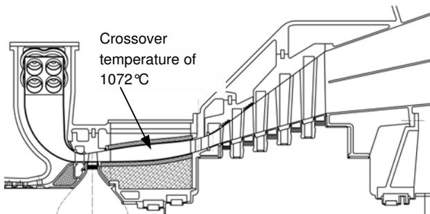
Figure 4 - Compressor turbine HTTC (8500 rpm) and crossover to power turbine HTTP (50 Hz).
