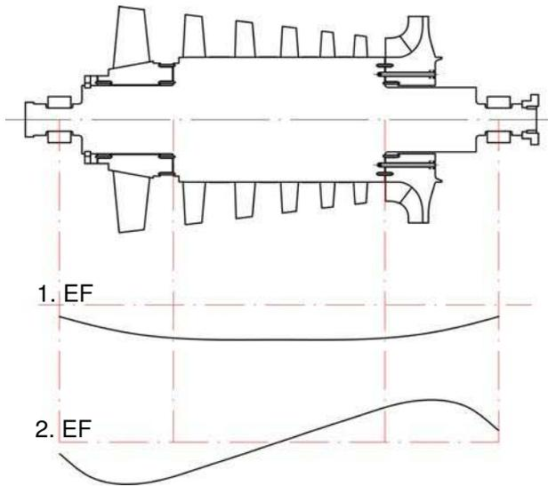
Figure 11 - Undamped eigenforms of rotor C1: First eigenform 88 Hz, second eigenform 280 Hz, operating speed 142 Hz.
