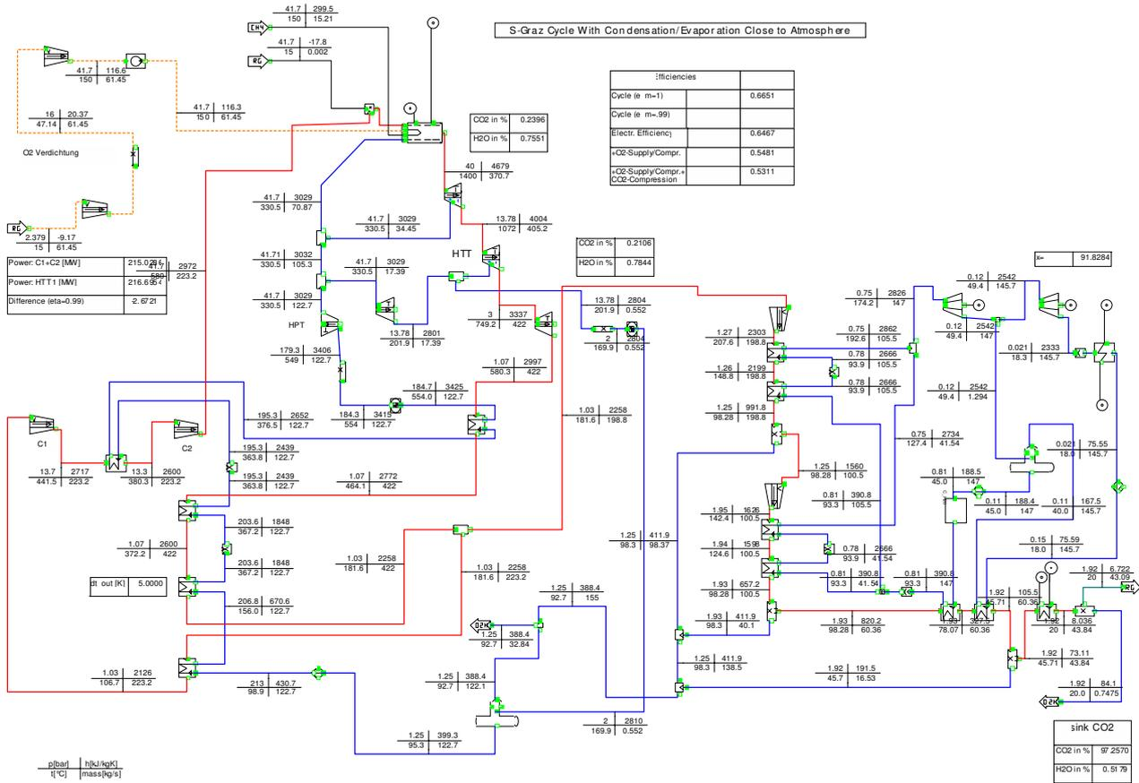
Figure 10 - Detailed thermodynamic cycle data of a 400 MW S-Graz Cycle Power Plant fired with methane
