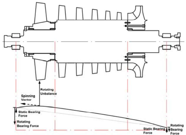
Figure 12 - Bearing amplitudes and rotor shaft bending of C1-HTTC rotor with foreign damage on blade tip of titanium blisk
