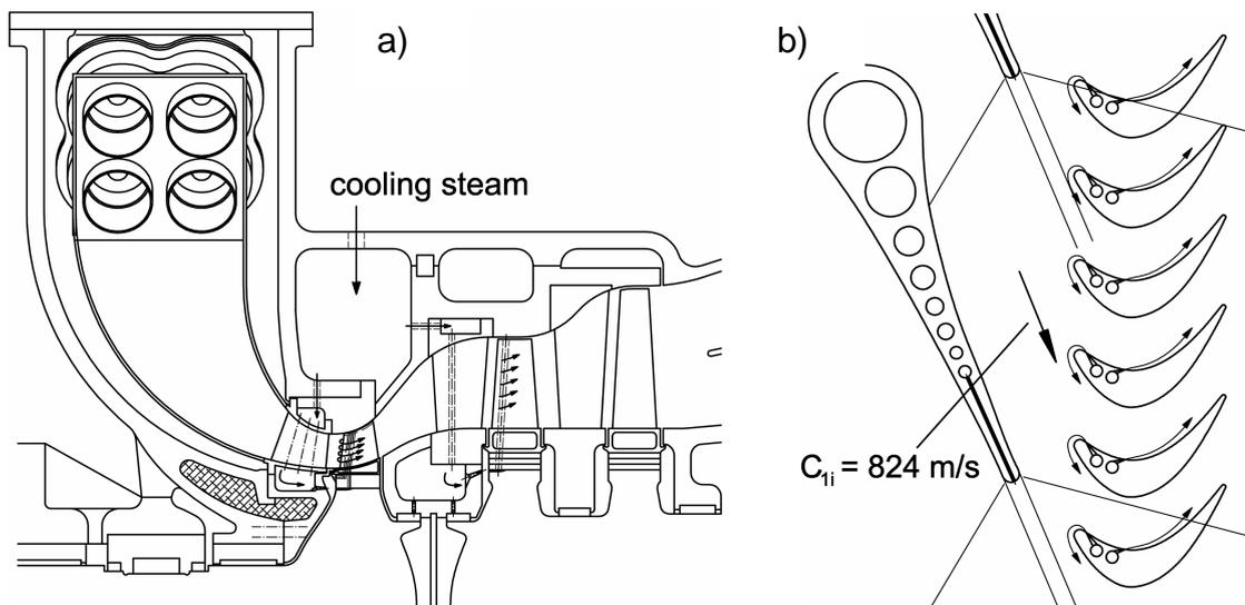
**Fig 4** a) HTT cooling flow in two stages and b) ICS cooling of first rotor blades
