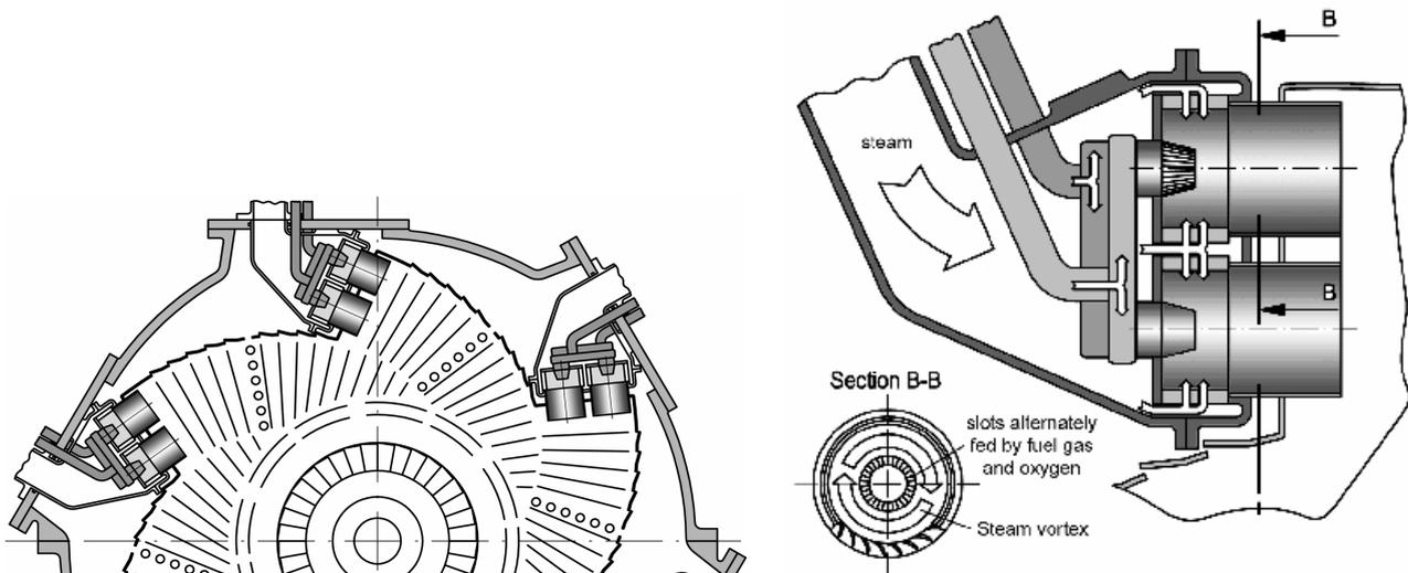
**Fig. 5** Combustion chamber and burner details
