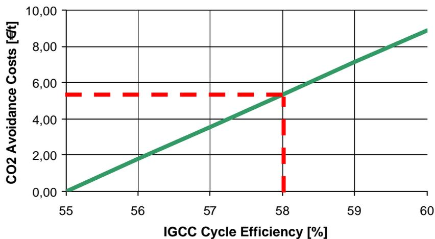
**Fig. 2** Sensitivity analysis of CO<sub>2</sub> avoidance costs vs. IGCC cycle efficiency
