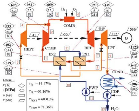
Fig. 1. Flow diagram and calculation results for the GRAZ cycle
