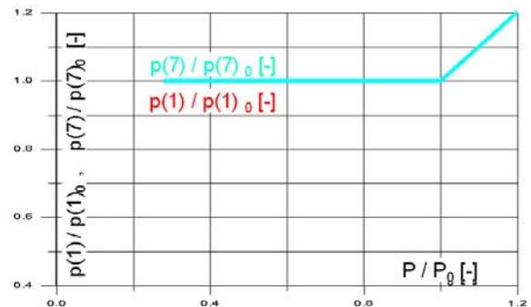
Fig. 8. The GRAZ cycle's part load characteristics (feed steam flow change): pressure vs. relative power
