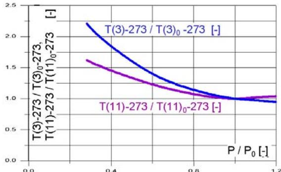
Fig. 10. The GRAZ cycle's part load characteristics (feed steam flow change): temperature vs. relative power
