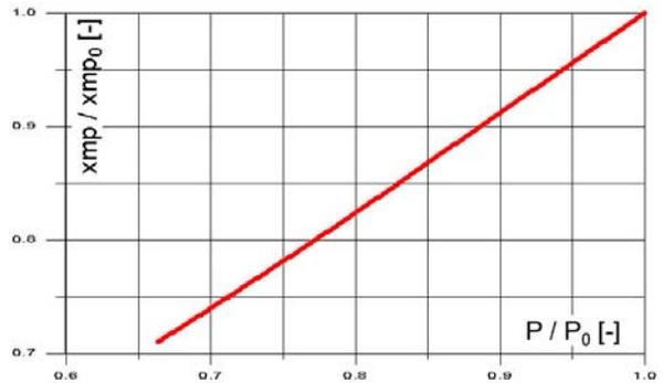
Fig. 15. The GRAZ cycle's part load characteristics (combustion temperature change): fuel mass flow vs. relative power
