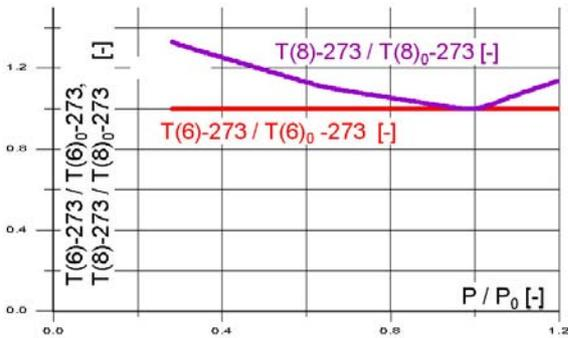
Fig. 11. The GRAZ cycle's part load characteristics (feed steam flow change): temperature vs. relative power
