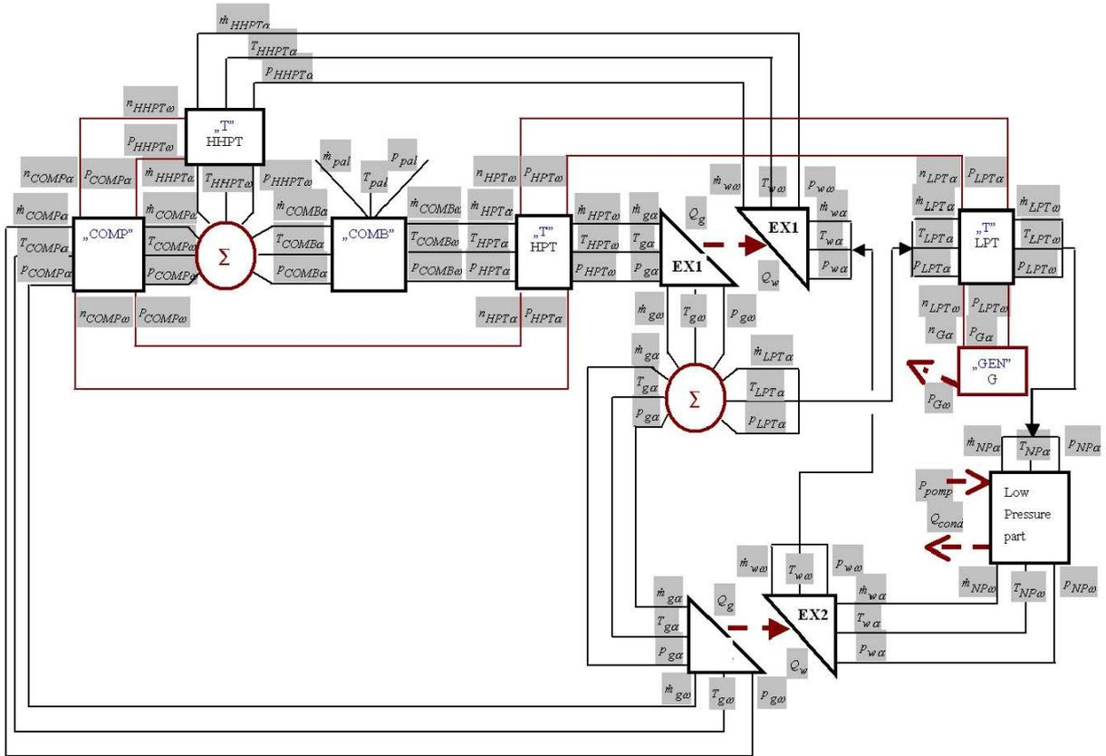
Fig. 2. Structure scheme of the Graz cycle's mathematical model
