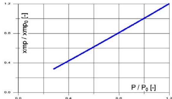
Fig. 7. The GRAZ cycle's part load characteristics (feed steam flow change): fuel mass-flow vs. relative power
