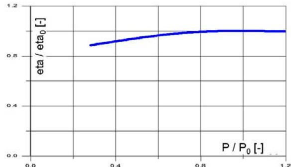
Fig. 6. The GRAZ cycle's part load characteristics (feed steam flow change): thermal efficiency vs. relative power
