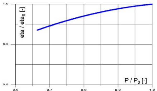
Fig. 14. The GRAZ cycle's part load characteristics (combustion temperature change): thermal efficiency vs. relative power
