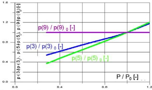
Fig. 9. The GRAZ cycle's part load characteristics (feed steam flow change): pressure vs. relative power
