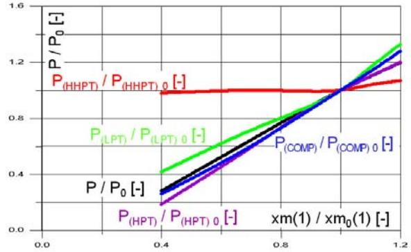
Fig. 5. The GRAZ cycle's part load characteristics (feed steam flow change): relative power vs. relative feed steam flow
