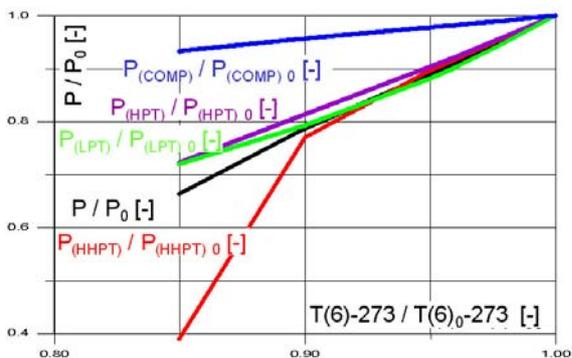
Fig. 12. The GRAZ cycle's part load characteristics (combustion temperature change): relative power vs. combustion temperature
