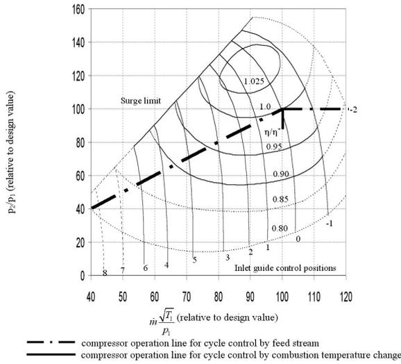
Fig. 4. Compressor characteristic: variable inlet vane angle
