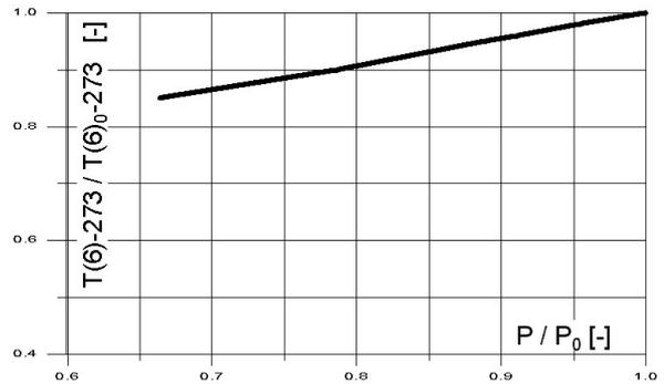
Fig. 13. The GRAZ cycle's part load characteristics (combustion temperature change): combustion temperature vs. relative power
